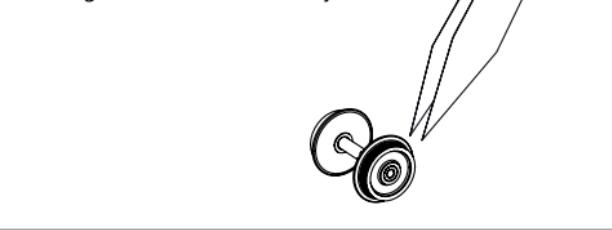
If used frequently, oil the wheelsets with a drop of non-resinous, acid-free sewing machine oil! In order to achieve the best possible running and traction properties, it is advisable to run the locomotive in forward for 25 minutes forwards and 25 minutes in reverse without load. Clean rails are essential for good performance.
